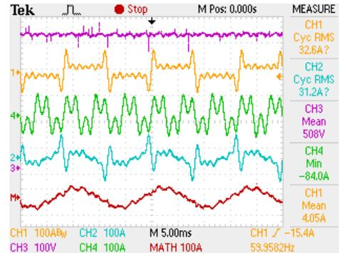
Figure 4. Harmonic currents generated and signals produce by active filter for 220 V prototype.
