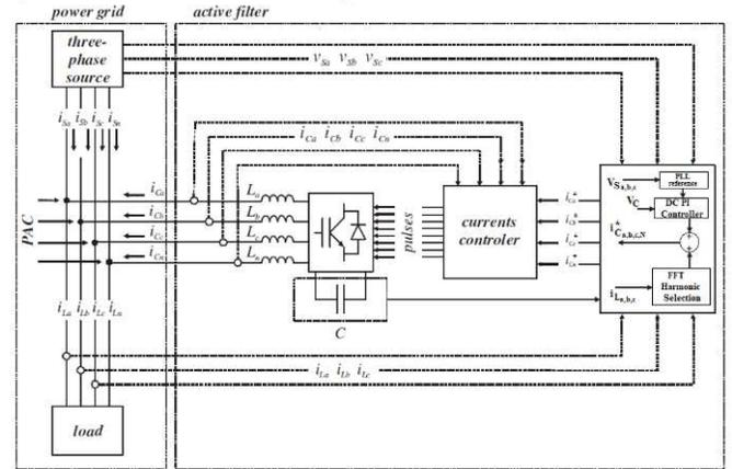
Figure 2. Topology used and general schematic of active filter hardware and control.
