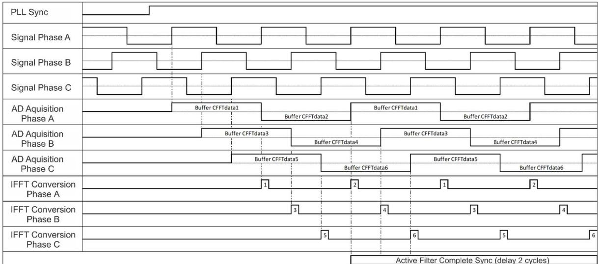
Figure 3. FFT and IFFT acquisition/processing methodology.
