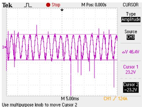
Figure 7. Oscillation voltage on busbar capacitor.
