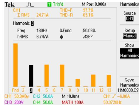
Figure 10. Harmonic current content for phase A.
