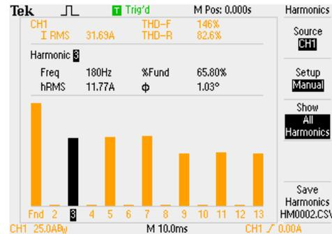
Figure 5. Harmonic current content for phase A.
