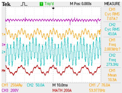
Figure 6. Harmonic currents generated and signals produce by active filter.
