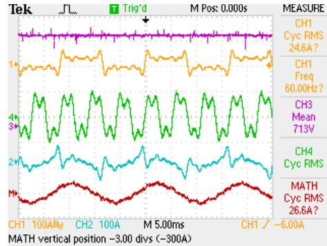
Figure 9. Harmonic currents generated and signals produce by active filter for 380 V prototype.
