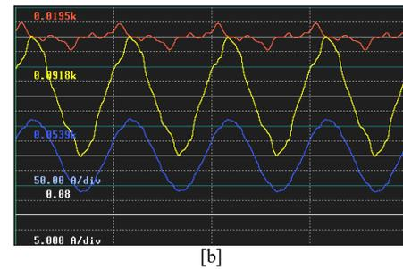
Figure 11. [a] Three-phase voltages and load currents; [b] Three-phase currents for 220 V unit at the BREE industrial plant.
