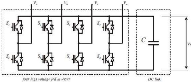
Figure 1. Voltage fed inverter with four legs [9].
