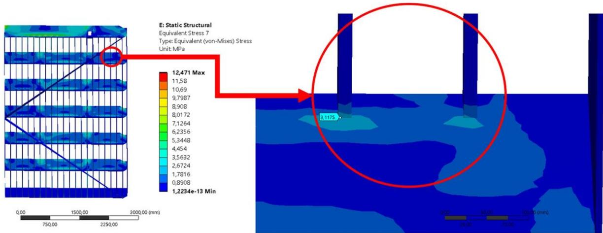
Figure 7. Result (mechanical stress) obtained by applying a weight force to the panel installed on the base plate. Partial result, prior to superposition with the stresses obtained by harmonic loading analysis.
