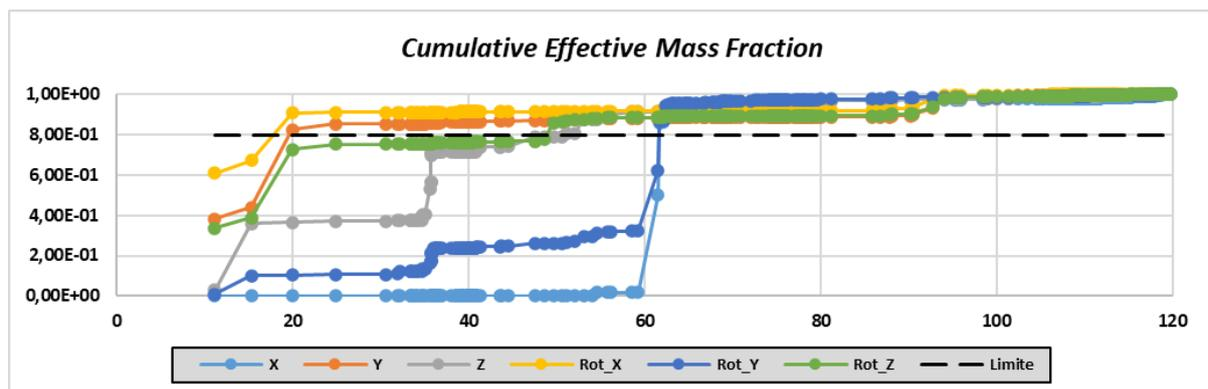
Figure 6. Plot summarizing the various natural frequencies of the structure (abscissa) and the ratio of the effective mass of each mode to the total mass of the structure (ordinate).
