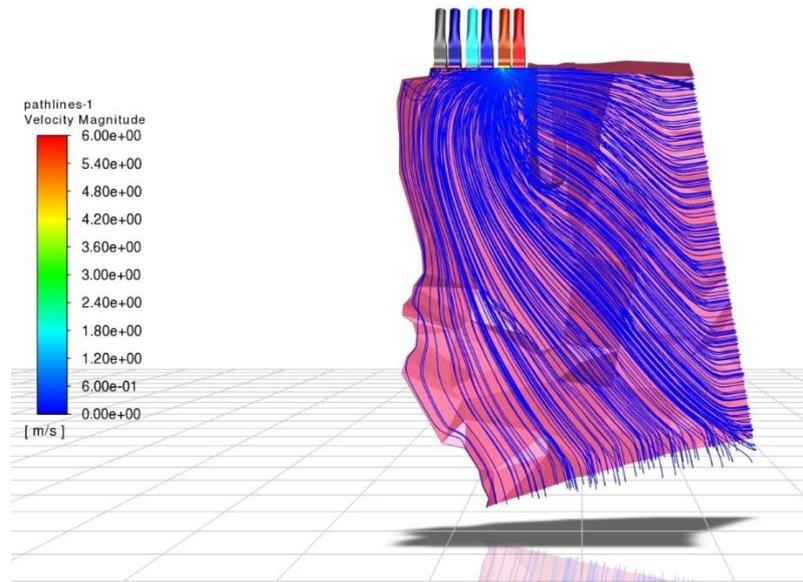
Figure 2. Geometry of a HPP reservoir and its velocity field, when operating with only 1 generating unit (GU).
