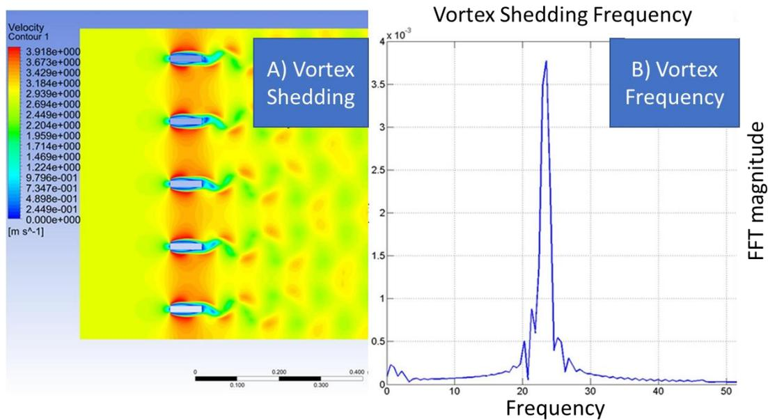
Figure 4. Velocity field (A) demonstrating the existence of alternating vortices and (B) the characteristic frequency of vortex shedding using FFT.
