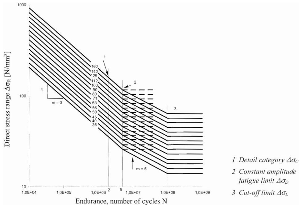
Figure 8. Direct stress range (MPa) as presented in Eurocode 3 for typical cases of welded joints.
