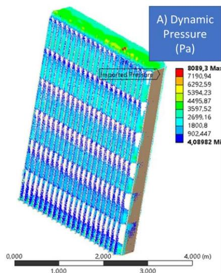
Figure 5. Dynamic pressure (Pa) passed to the structural model. Result obtained from CFD.
